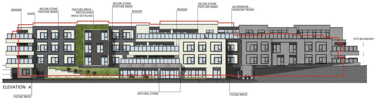
Further elevational differences highlighted as follows, extracts show: 'Elevation A' as the western/frontage elevation; 'Elevation E', which is the southern block facing Paradise Walk that has increased from three to four storeys; and 'Elevation F' which is the same block as facing the rear of properties on Sparkhays Drive >35m away.
